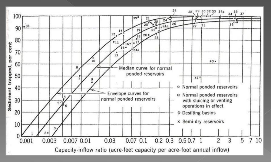
• The figure may be utilized to estimate the amount of sediment a lake/reservoir will trap if the average annual sediment load of the stream/s is known. The volume occupied by the sediment can be computed, using a reasonable value of specific weight for the deposited sediment.
